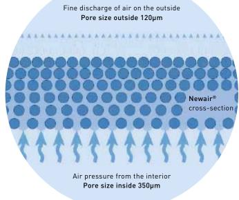
The newair aerator is characterized by a special material structure. The size of the pores reducing in flow direction. On the one hand there will be created a huge upstream flow area for the air, on the other hand there will be reached a fine allocation of the bubbles by a small pore size on the outlet side.
